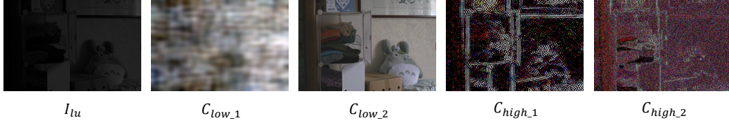
Figure 4: The visualization of the five image priors. They represent chromaticity, semantic information, edge contours, and noise intensity.
