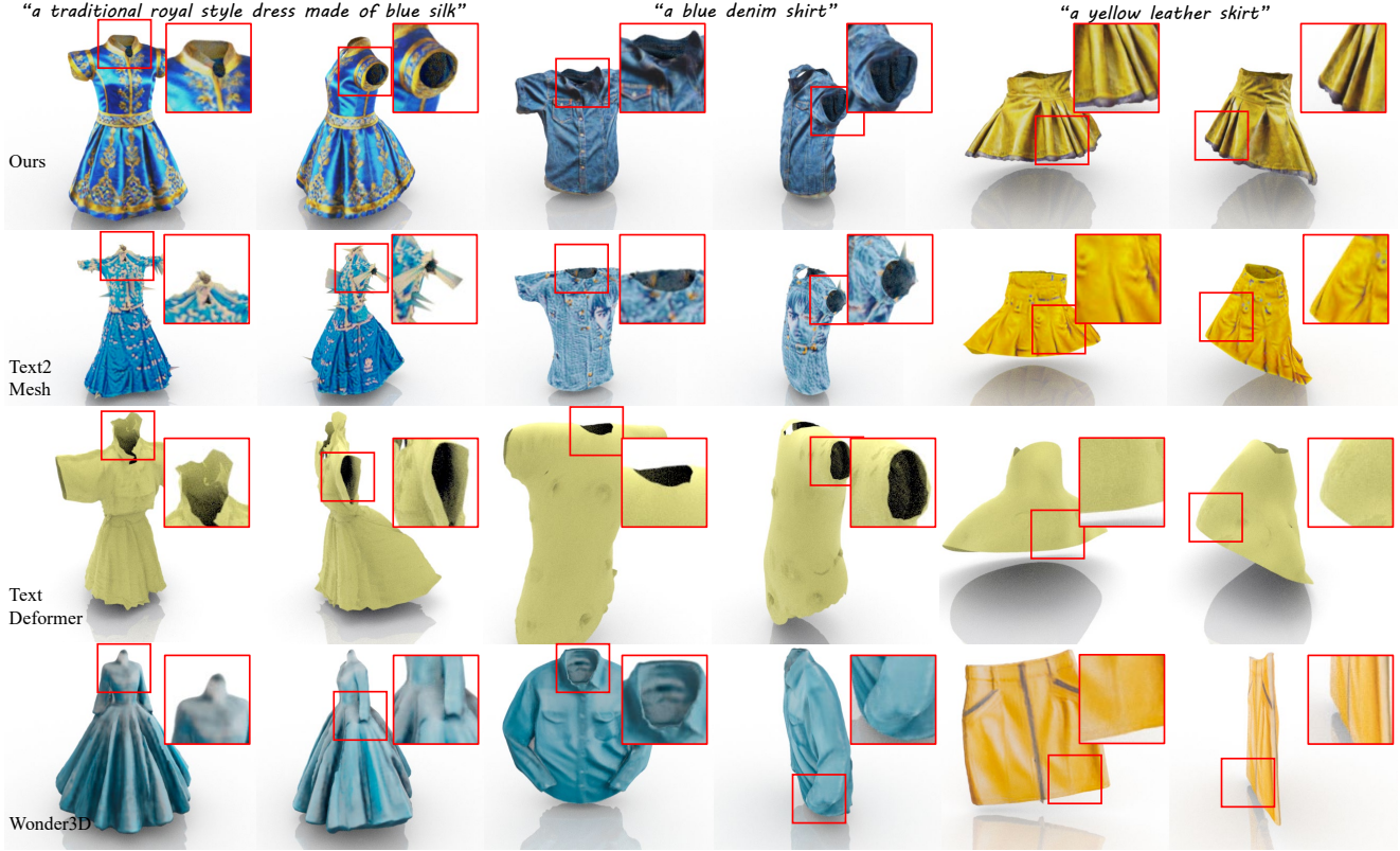
Figure 3. Qualitative Comparisons. While baseline methods either produce unrealistic geometric artifacts, e.g. spikes and excessive smoothness, or non-garment textures, GarmentDreamer excels in generating high-quality, simulation-ready non-watertight garments with detailed textures and fine wrinkle details.
