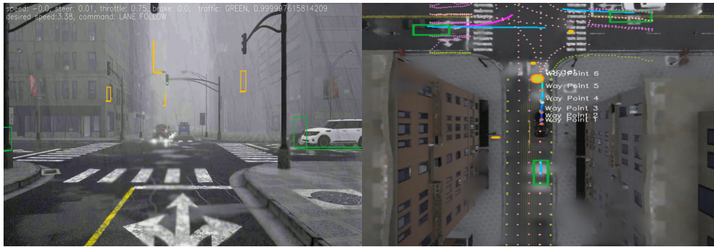
(g) Traffic light recognition under rainy weather conditions
