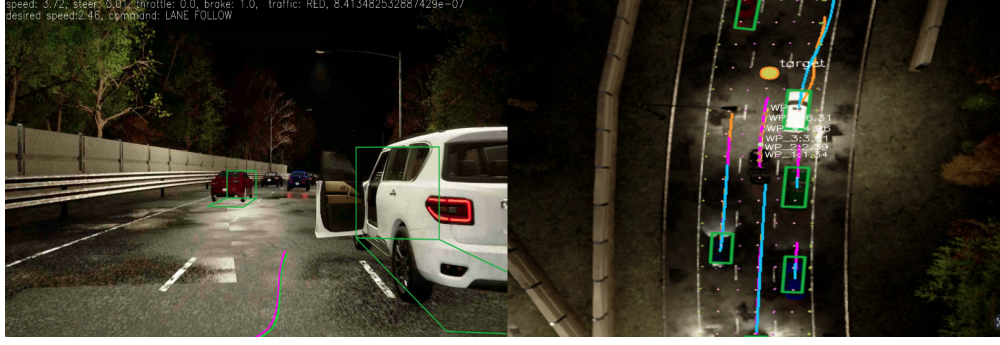
(a) Failure to avoid a vehicle with an opened door.
