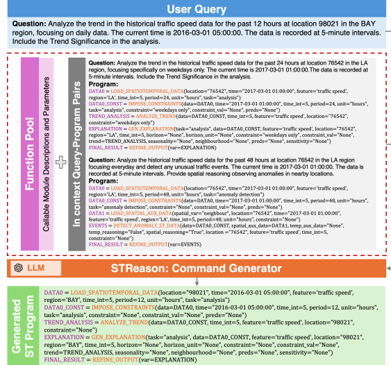
Figure 2: STReason Command Generator uses a Function Pool and in-context query-program pairs to generate executable ST-Program for a given user query.
