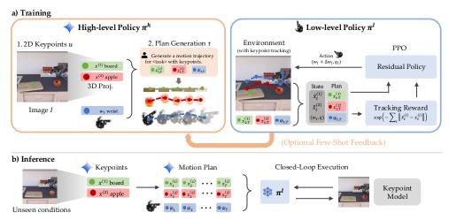
**Figure 2:** a) Training: a high-level VLM predicts 3D keypoint plans, which a low-level policy learns to track via RL. b) Inference: new plans are generated by the VLM, which are executed by the frozen low-level policy.
