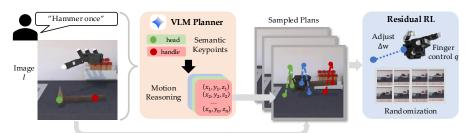
**Figure 1:** Overview of our method: a VLM generates hand and object keypoint trajectories from a language command and scene image. A low-level residual RL policy is trained to track these trajectories in simulation.
