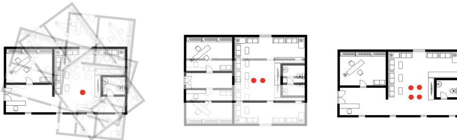
Figure 4: Ambiguity exists in acoustic measurement due to the omni-directional nature of our sensor. (a) rotational ambiguity for a single measurement. (b) flipping ambiguity for two measurements. (c) we use four measurements for one estimation to resolve ambiguity.
