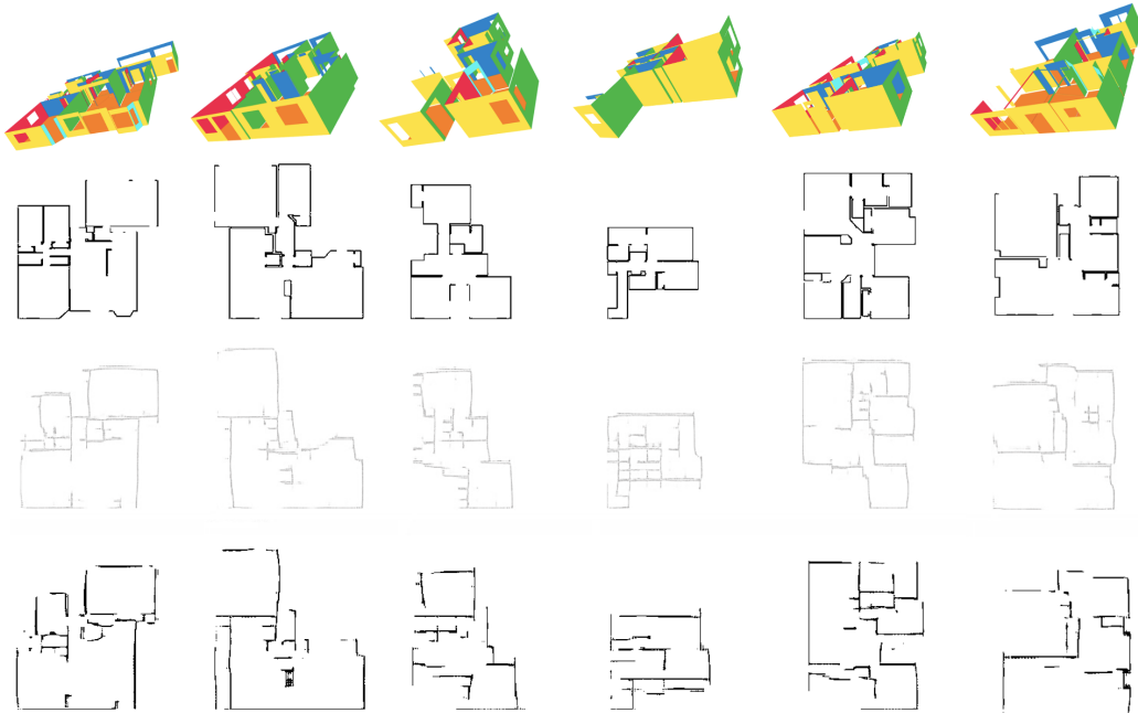
Figure 10: Qualitative results for MapLearn on simulation data. Row (a) 3D mesh of experimental environment, (b) floor plan ground-truth, (c) floor plan estimation for ablation study, hint map only, (d) floor plan estimation for MapLearn.
