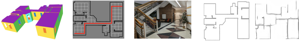
Figure 1: (a) 3D mesh of simulation environment, (b) an example trajectory, (c) real world experimental environment, (d) groundtruth floorplan, (e) estimation result.
