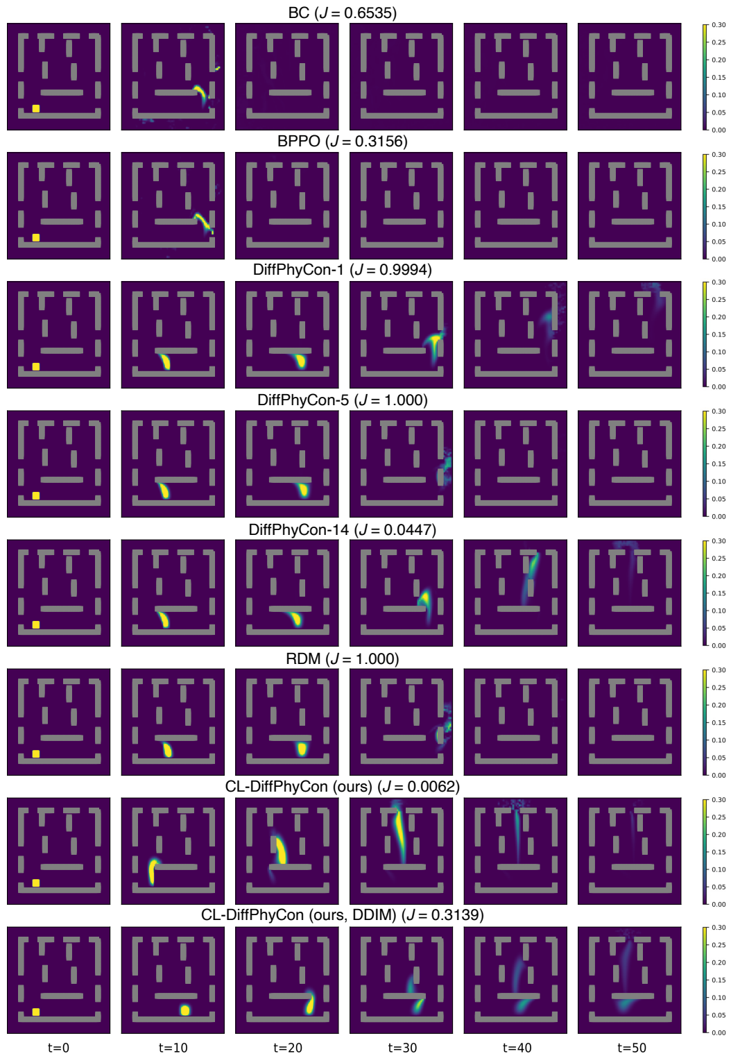
Figure 15: Visualizations results of 2D fluid control by our CL-DiffPhyCon method and baselines for the same test sample. This is an example of the random map setting. Each row shows six frames of smoke density. The smaller the value of J , the better the performance.
