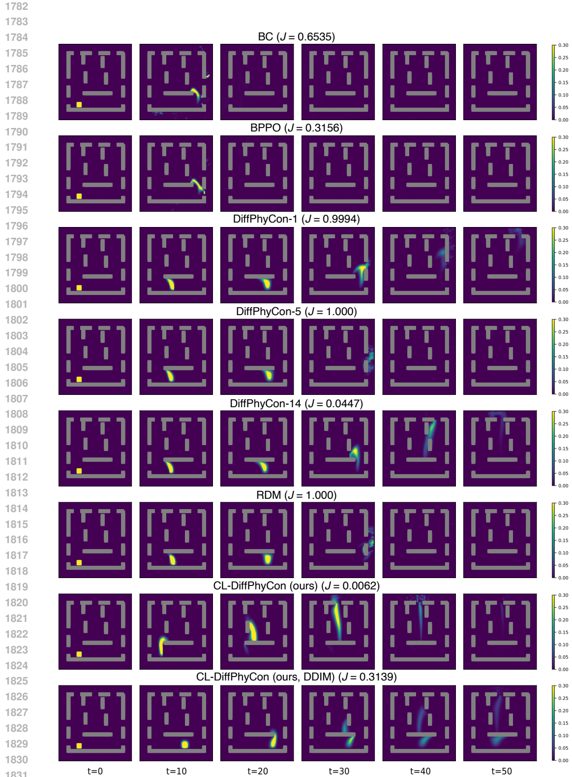
Figure 15: Visualizations results of 2D fluid control by our CL-DiffPhyCon method and baselines for the same test sample. This is an example of the random map setting. Each row shows six frames of smoke density. The smaller the value of J , the better the performance.
