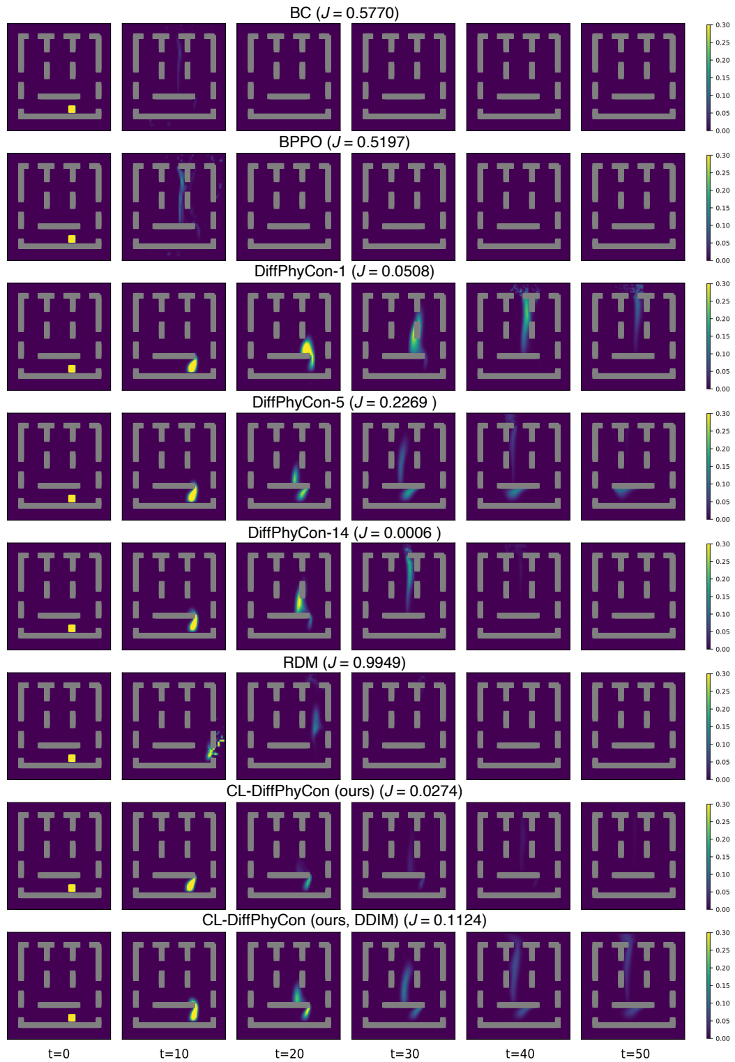
Figure 13: Visualizations results of 2D fluid control by our CL-DiffPhyCon method and baselines for a same test sample. This is an example of the fixed map setting. Each row shows six frames of smoke density. The smaller the value of J , the better the performance.
