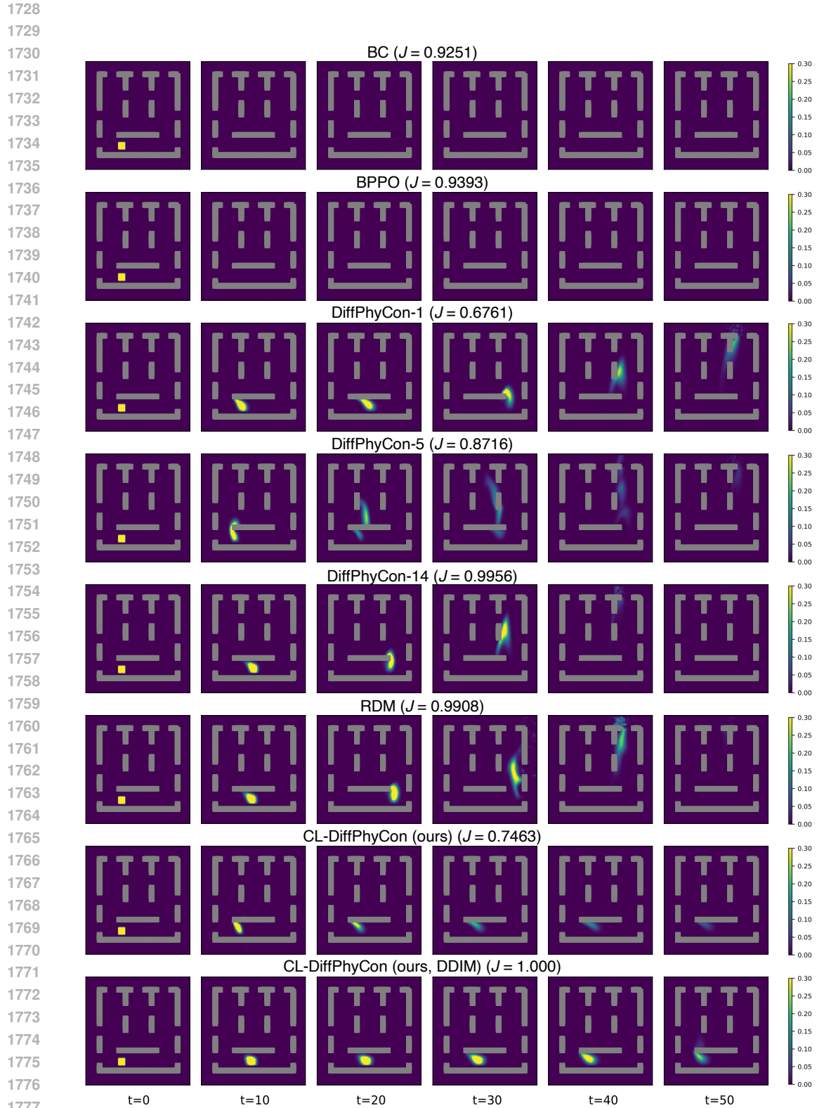
Figure 14: Visualizations results of 2D fluid control by our CL-DiffPhyCon method and base-lines for the same test sample. This is an example of the fixed map setting. Each row shows six frames of smoke density. The smaller the value of J , the better the performance.
