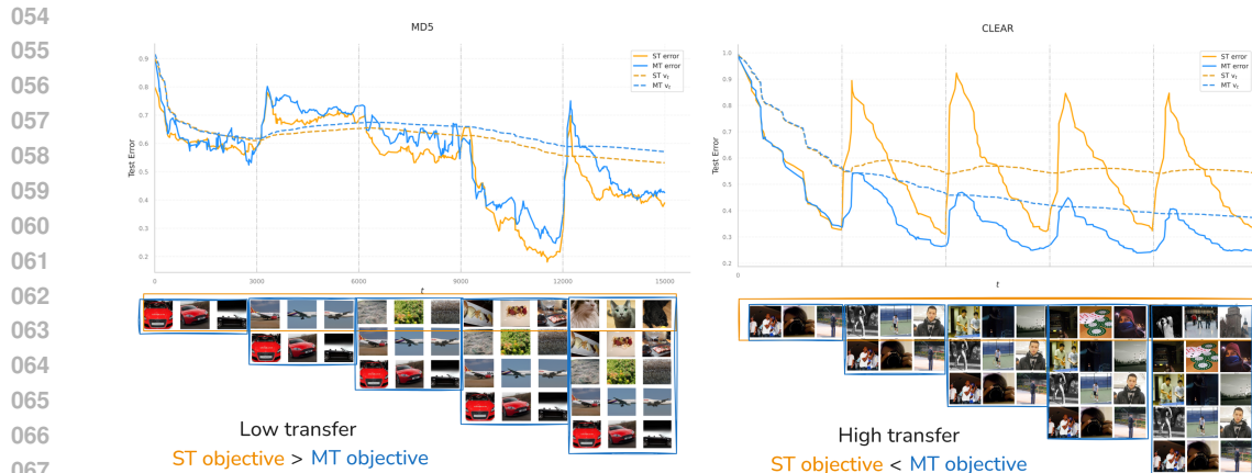
Figure 1: Diagram depicting the potential sub-optimality of the multi-task objective depending on the data distribution. On the right, a data stream is selected such that multitask objective (blue) outperforms single task learner (orange), while on the left the reverse is true. In section 4 we will formalize this behaviour, and in section 5 we will argue that CL algorithms can estimate in which condition they might be and adapt to it.
