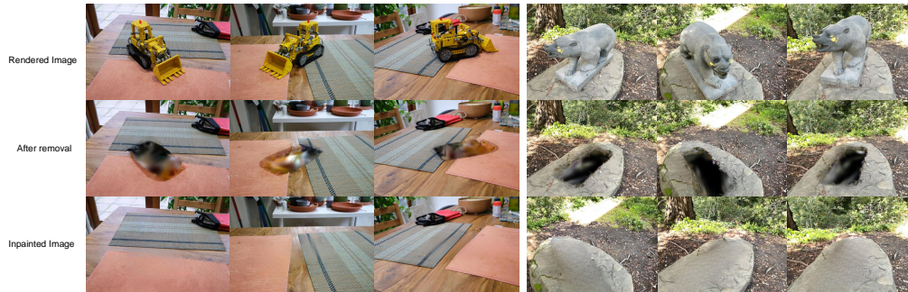
822 Figure 8: 3D object Inpainting of our method. We use LAMA (Suvorov et al., 2022) to inpaint the 823 images after object removal, and then finetune Gaussians based on the inpainted 2D images. 824
