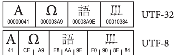
Figure 2: Comparison of variable width Unicode encoding (UTF-8) and fixed width encoding (UTF-32). Image adapted from (The Unicode Consortium, 2022).
