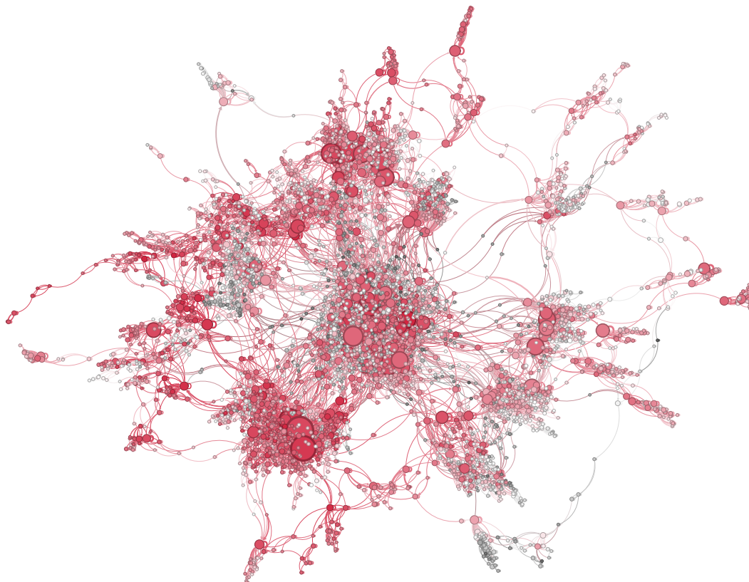
Figure 9: Visualization of the local optima network of NAS-Bench-101 test landscapes at the 108- th epoch, containing 5,908 nodes. Radius of each node (i.e., local optimum) indicates size of the corresponding basin of attraction. The color indicates test accuracy, where warmer color is better. Edges indicate transition probabilities between local optima, where thicker, warmer edges imply the corresponding transition is more likely to happen. Edge directions indicate the improving direction (i.e., pointing to the fitter configuration).
