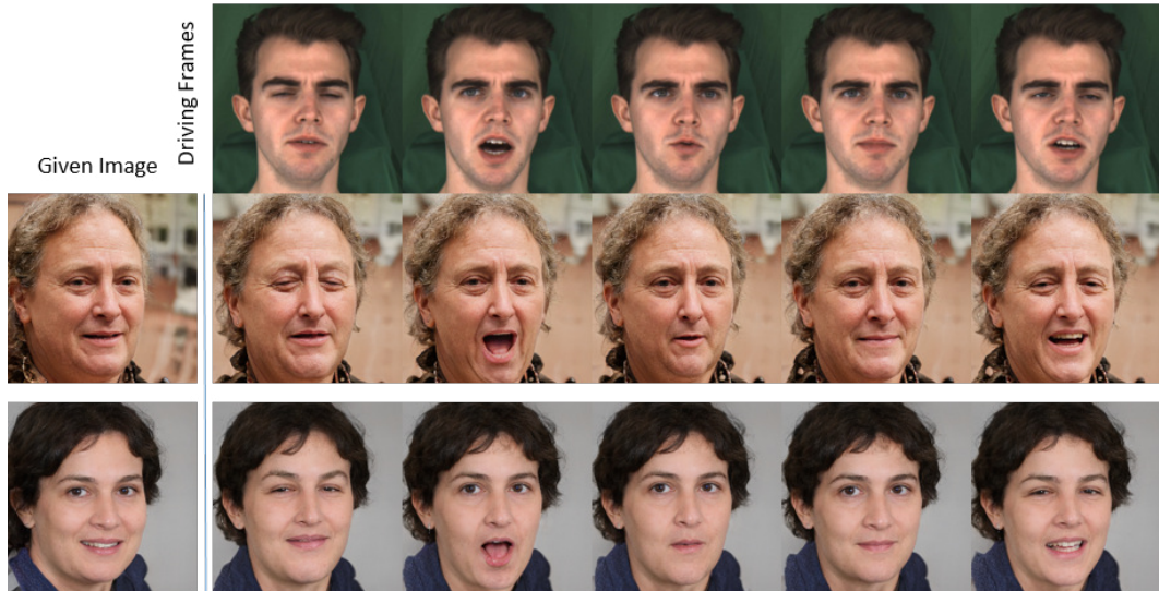
Figure 6: Editing global pose and expressions. Given a reference image and a driving frame, we match the pose and expressions. Each row shows an identity (reference image) and edits corresponding to the top row (driving frame).
