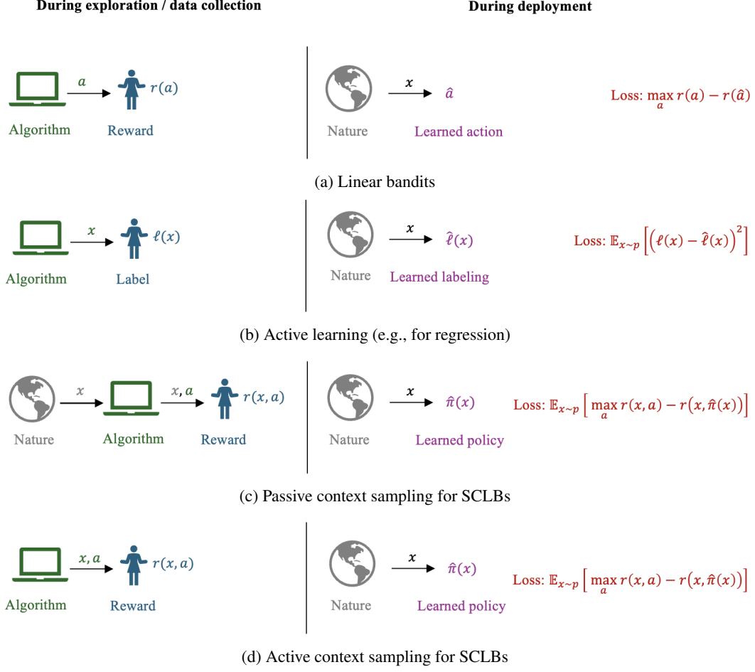
Figure 4: Four learning paradigms. Figure 4a describes the typical linear bandit setting, where there are no contexts and the learner’s goal is to learn a good universal action. Figure 4b shows active learning for regression, with the mean-squared loss. During exploration, the learner actively samples data x to learn a label function \hat{\ell}(x) ; but during deployment, inputs arrive according to the distribution p . In other settings, such as active learning for classification, this mean-squared loss might be replaced with another smooth, convex loss function. In contrast, in contextual bandits (Figures 4c and 4d), the learner needs to learn a policy-to-action mapping. In this case, the loss function is the sub-optimality of the policy—which is discontinuous—and consequently, traditional techniques from continuous optimization do not immediately apply.
