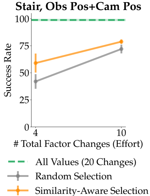
Fig. 14: Performance of the Stair strategy for the Pick Place task, when composing object position and camera position . We find that selecting factor values using a similarity-aware strategy outperforms random selection (as done in our main simulation results).
