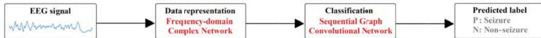
Fig. 3. Workflow of our epilepsy detection framework, with frequency-domain complex network and Sequential Graph Convolutional Network (SGCN) as its key design features.
