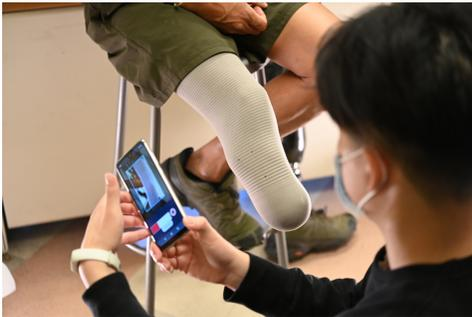
Figure 1: Scanning a Transtibial Amputee using the Lim(b)itless Cell Phone Application
