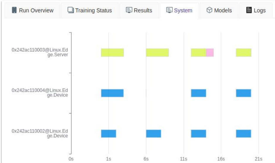
Figure 13: Deployment Interface Example of FedML-HE: Overhead distribution monitoring on each edge device (e.g. Desktop (Ubuntu), Laptop (MacBook), and Raspberry Pi 4), which can be used to pinpoint HE overhead bottlenecks and guide optimization.
