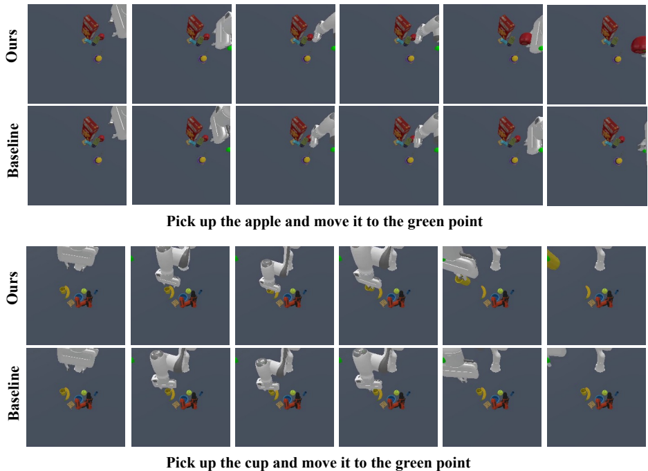
Figure 4: Visualized comparison between Diffusion Transformer Policy and Diffusion Action Head baseline on Maniskill2 (PickClutterYCB). The first row is Diffusion Tranformer Policy, while the second row is the baseline method with Diffusion Action Head.
