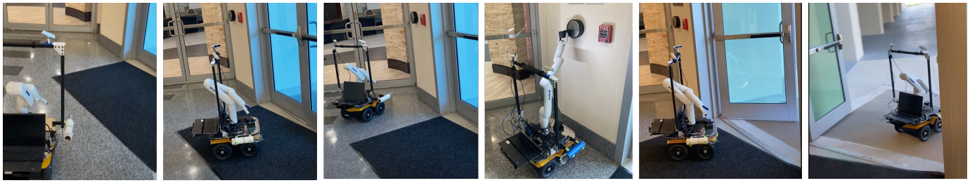
Fig. 10: Representative sequence of one navigation task. From left to right: (1) Following a planned path. (2) Blockage encountered. (3),(4) Reasoning and executing unblocking solution. (5) Path cleared. (6) continuing and completing the navigation task.
