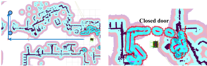
(a) Initially planned global path. (b) Blockage discovered near the destination; navigation fails.
