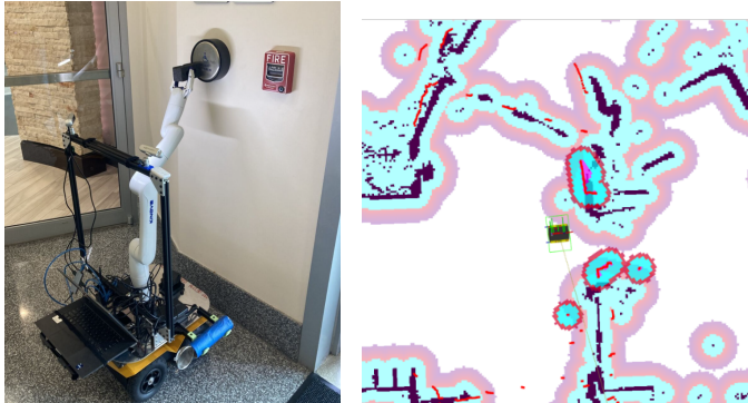
(a) With the blockage reasoning, the robot detects and click the door button to unblock itself. (b) The map shows an opened space after clicking the door button.
