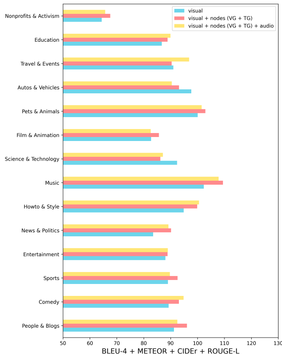
Figure 3: Sum of BLEU-4, METEOR, CIDEr and ROUGE-L scores for the ActivityNet predicted captions across the different video categories using 3 different input modalities (visual only, visual + nodes, visual + nodes + audio). The scores are obtained from the combined validation ( ae-val ) and testing set ( ae-test ).
