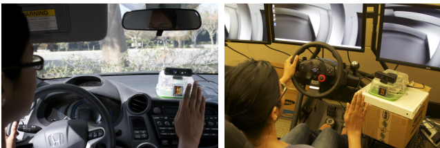
Fig. 7: Experimental setup. We used two different experimental setups for gesture data acquisition, i.e. , outdoors in a real car (left) and indoors in a driving simulator (right).
