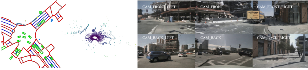
Figure 7: Joint generation of LiDAR and multi-view video. Our method generates spatially aligned LiDAR and camera views conditioned on a shared right turn T-junction layout.
