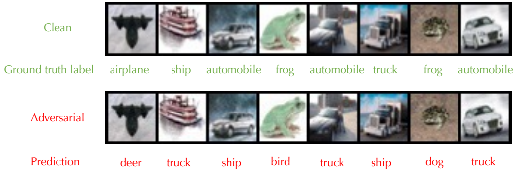
Figure 5: Visualization of the clean images and adversarial samples generated by DiffAttack on CIFAR-10 with \ell_\infty attack ( \epsilon = 8/255 ) against score-based purification with WideResNet-28-10.
