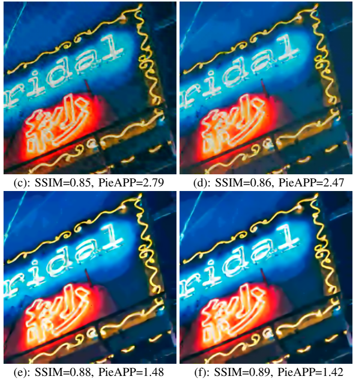
Fig. 11. (a) Original test image (image 3 of the CLIC dataset). The reconstructed ones at 0.2 bpp using: (b) JPEG2000, (c) CNN-LS [23], (d) FCNN-LS-JL-SL [25], (e) FCNN-LS-JL-ML1, (f) FCNN-LS-JL-ML2.
