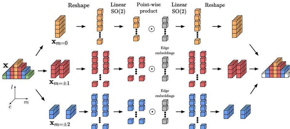
Figure 6. The  $SO(2)$  block for  $L = 4$ ,  $C = 4$  and  $M = 2$ . The orange, red, blue and green shaded entries are the coefficients of the spherical harmonics of  $m = 0, 1, 2$  and  $3$  respectively.
