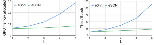
Figure 1. We implement two mathematically equivalent equivariant GNNs. *e3nn* uses the e3nn PyTorch library, whereas *eSCN* uses our novel approach. **Left:** GPU memory allocated (%) at training time with respect to the maximum degree of the spherical harmonics ( $L$ ). **Right:** time (h) per epoch by  $L$ . We fix the number of channels to  $C = 64$  and remove any non-linearity.
