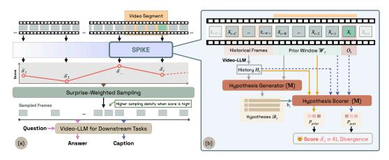
Figure 2: (a) Overall architecture: SPIKE computes surprise scores, which guide weighted frame sampling for downstream tasks. (b) SPIKE: Given history  $H_t$ , prior window W, and observed frame  $O_t$ , the hypothesis generator produces belief set  $B_t$ . The hypothesis scorer computes  $P_{prior}$  and  $P_{post}$ , yielding surprise score  $S_t$  as KL divergence.
