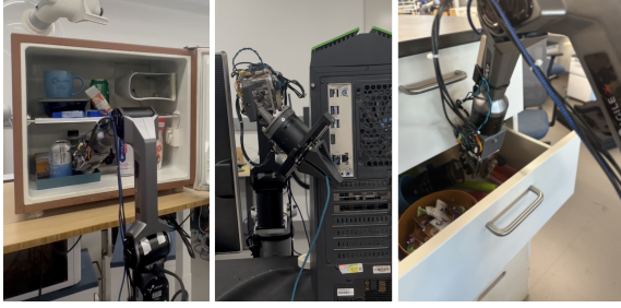
Fig. 5: The three tasks shown to evaluate the performance of the wrist as compared to the stock AgileX arm.
