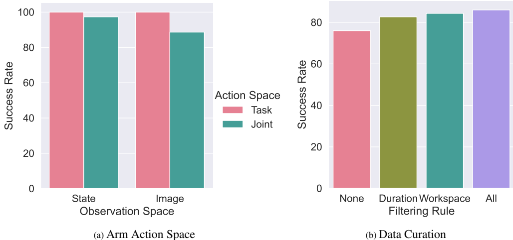
Figure C.1: Effect of Arm Action Space Choice and Data Filtering Rules. (a) OPTIMUS task success rate improves with task-space over joint-space actions when using image observations. Image observation-space policies perform comparably to the privileged state-based policies when using task-space actions. (b) Performance is improved by filtering TAMP success trajectories based on the visible workspace and their duration.
