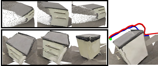
Figure 9: Single-image extraction leaves occluded regions incomplete, VGER reliably reconstructs them. Left: Top: DepthAnythingV2; bottom: VGER.; Right: Trajectories approaching the cabinet from the occluded backside, avoiding collision to reach the green goal.
