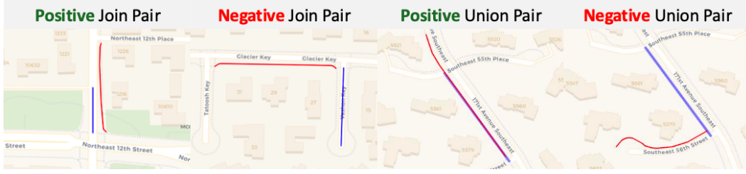
Figure 1: Positive and negative examples for the spatial join and union task. (1) For the spatial join task, the blue line represents the road, and the red line represents the sidewalk. The task classifies whether a sidewalk “runs alongside” a road from a pedestrian’s perspective. (2) For the union task, both lines represent sidewalks. The task determines whether two sidewalks fully or partially represent the same real-world entity.
