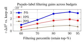
(a) Accuracy gains vs. filtering strength. Gains peak near the 90th percentile at 5–10% labels, then taper as label budgets increase.
