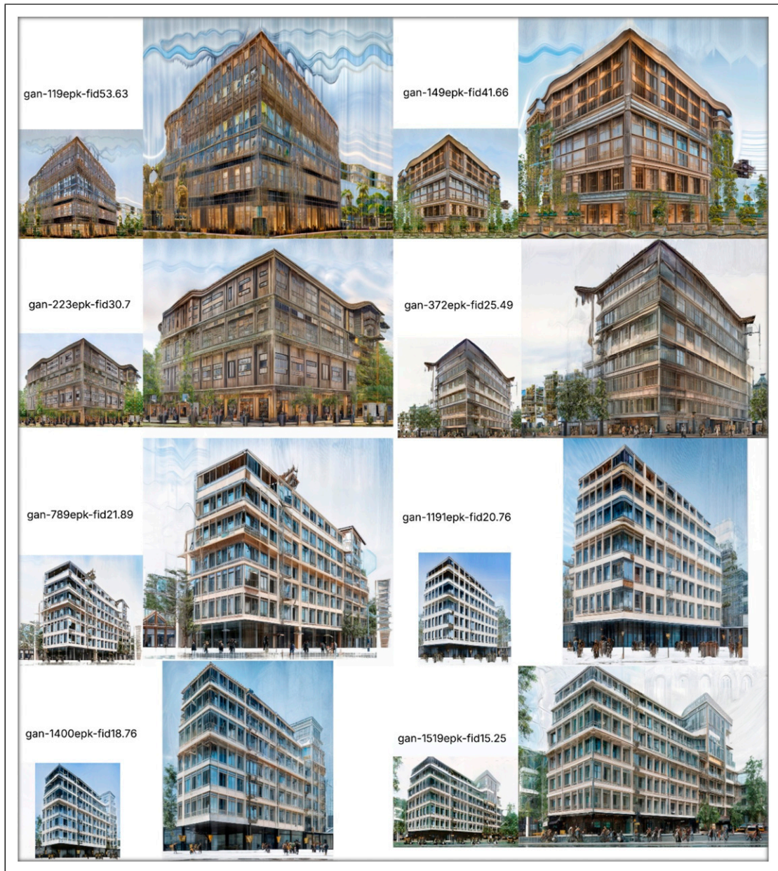
Figure 7. Starting from the same random seed, this series shows the progression of StyleGAN2-ada quality and KREA interpretation, as a function of the number of training epochs (epk) and the associated FID. Clearly, below the FID=30 threshold, results improve markedly and become credible.
