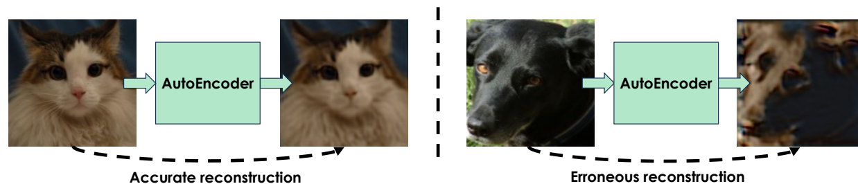
Figure 2: Autoencoder Reconstruction Error An autoencoder trained exclusively on cat images yields accurate reconstructions on other cat images (left) and inaccurate ones on dog images (right). Thus, the distance between an image and its reconstruction can be used to estimate whether that image is likely to be a cat image or not.
