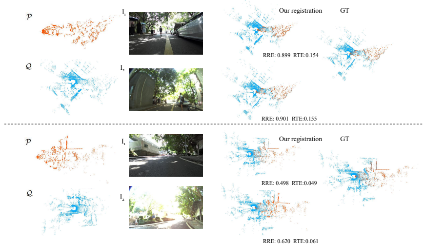
Figure 11: The visualization registration result by using a distorted and overexposed image captured from the RGB camera with different installation position.
