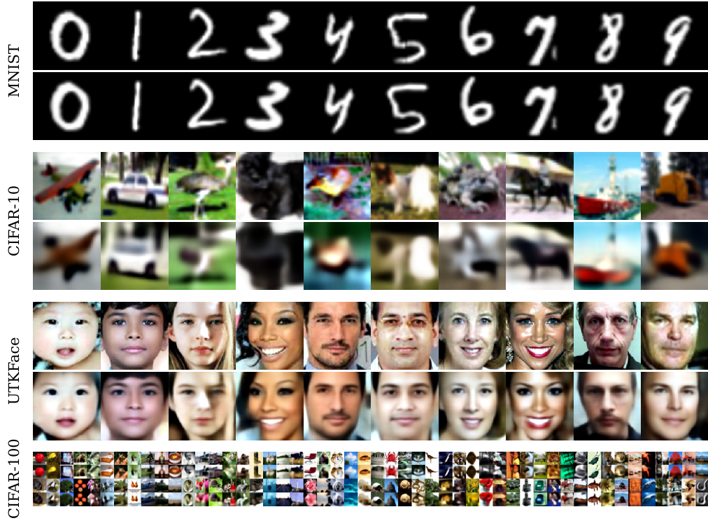
Figure 8: WAE reconstruction comparison on natural images datasets. For each dataset, the upper image is the input, while the lower is the reconstruction.
