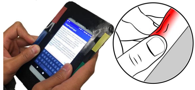
Figure 1: BendAide is a 3D printed case that is fitted around a touchscreen mobile device. Its deformable bezel detects bend input, providing an alternative interaction modality to touch in support of complex text tasks.
