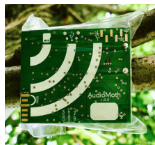
Figure 8: An AudioMoth deployed to listen for the presence of cicada species in the New Forest National Park, UK
