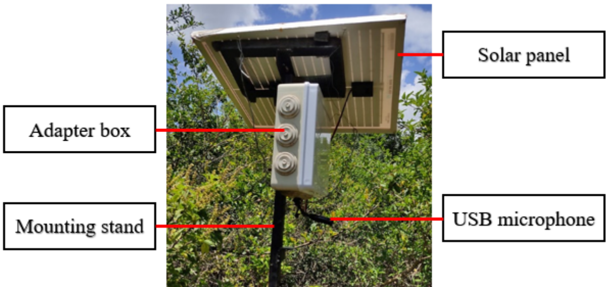
Figure 3: The DSAIL Bioacoustics System deployed at the Dedan Kimathi University of Technology Conservancy for acoustic data collection.
