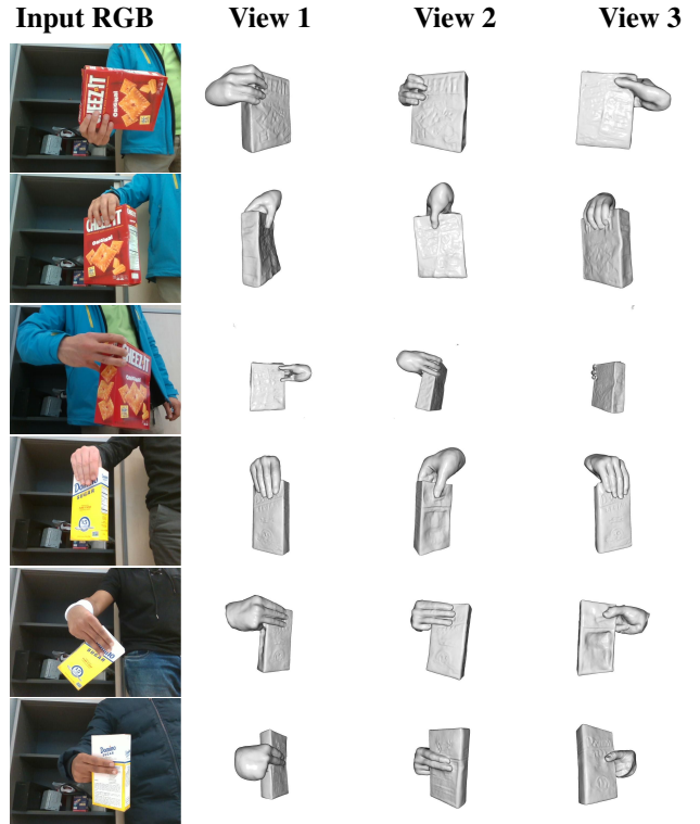
Figure 1. Qualitative Hand-Object reconstructions on the HO3D dataset. The first column is an RGB frame of the input sequence, followed by 3 different views of the reconstructed hand-object shape using HOS t 3R, our proposed method.
