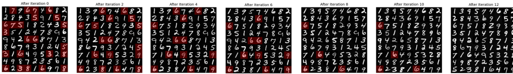
Figure 1: Progressive refinement on MNIST Sudoku with IPR. From left to right, Iterative Partial Refinement (IPR) progressively corrects erroneous cells (highlighted in red), resolving global constraint violations and converging to a valid Sudoku solution.
