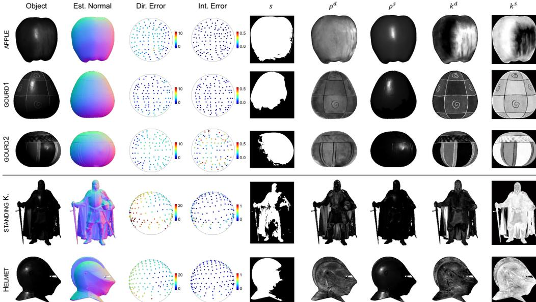
Figure 4: From left to right: the reference image, estimated surface normal map from our method, the lighting direction error, light intensity error, the estimated shadow map, diffuse reflectance map, specular reflectance map, diffuse scaling coefficient map, and specular coefficient map. Top three objects are APPLE, GOURD1, and GOURD2 from APPLE & GOURD dataset [2], and bottom two objects are STANDING KNIGHT and HELMET from LIGHT STAGE DATA GALLERY dataset [11].
