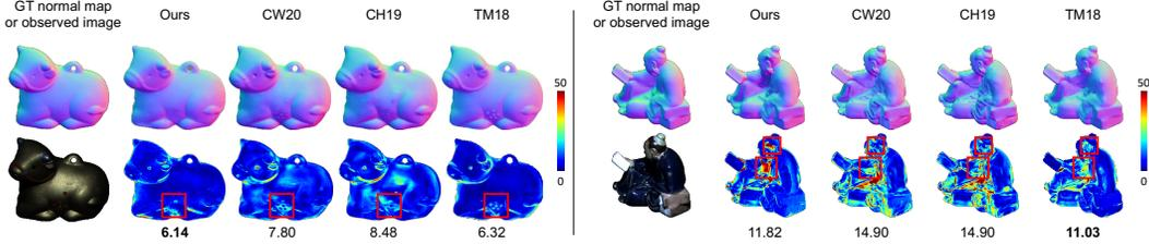
Figure 3: Visual quality comparison in terms of normal map and error map on COW (left) and READING (right) from DiLiGENT [45]. For each subfig, from left to right: ground truth of normal map or observed image, normal map / error map from our method, CW20 [15], CH19 [13], and TM18 [47].
