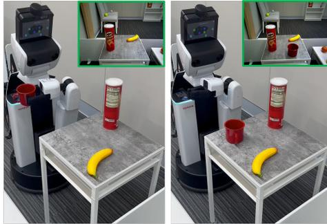
Figure 3: Experimental environment. The left and right images show the state before and after manipulation, respectively. Instruction sentences, such as “place a mug in front of the banana,” were created based on the situation before the manipulation. Examples of the egocentric images are shown at the top right of each exocentric image.
