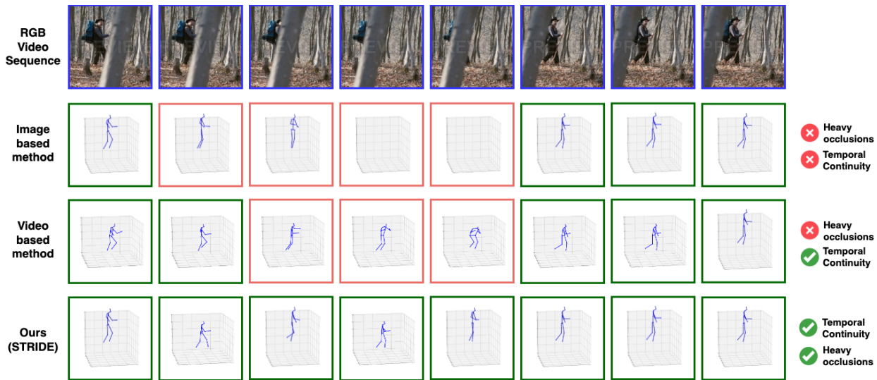
Figure 1. Effect of occlusions on pose estimation. Image-based 3D pose estimators [3] often struggle with heavy occlusions, as illustrated in this figure. Without temporal context, predictions on highly obscured frames are inconsistent with prior poses, like the erroneous pose in the third column. Notably, even state-of-the-art video approaches [36] fail on prolonged full occlusions spanning multiple frames, as in columns 4 and 5. This highlights yet another critical limitation - models are brittle when deployed outside their training distributions. Without training examples of such long-duration occlusions, models fail to extrapolate reasonable poses. Our work addresses this through test-time training of a human motion prior. By fine-tuning on each new video, we tailor this parametric prior to handling sequence-specific occlusion patterns not observed during training. Given an initial noisy estimate, our approach refines the pose sequence into an accurate, temporally coherent output, as shown in the final row.
