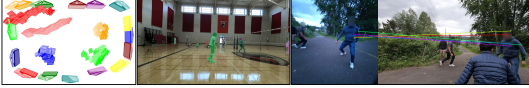
Figure 12: Failure Case Visualizations We visualize failure cases across our camera pose, motion segmentation, and spatial correspondence modules. Specifically, observe the incorrect predicted camera poses for the dynamic camera (red) against the ground truth (pink). Background individuals are occasionally mis-segmented for motion segmentation, and some segmentations appear fragmented. Furthermore, Mast3R sometimes generates incorrect correspondences within dynamic masks.
