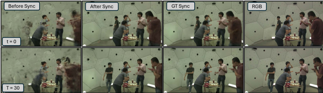
Figure 7: K-Plane Rendering on VisualSync Results. We train K-Planes on CMU Panoptic [22] multi-view videos for novel view synthesis. Unsynchronized inputs (1st) produce blurry results, while our synchronized outputs (2nd) are sharp and comparable to ground-truth sync (3rd). The 4th column shows real images. Our method enables high-quality synthesis from unsynchronized inputs.
