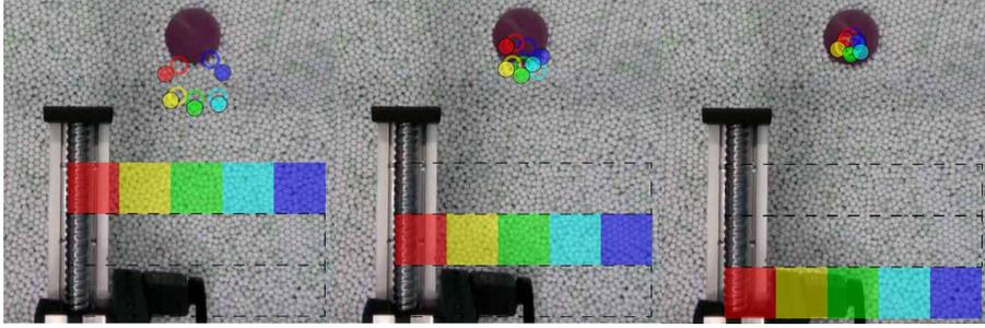
Figure 5: Obstacle movement with different excavation actions, visualized with colored squares (5 actions per image above). These  $5 \times 3 = 15$  colored squares are the 15 discretized excavation actions we consider. The corresponding *solid* color circles and *empty* color circles are the trained model’s predicted obstacle positions and experiment-measured obstacle positions, respectively. (This figure is best viewed zoomed-in.)
