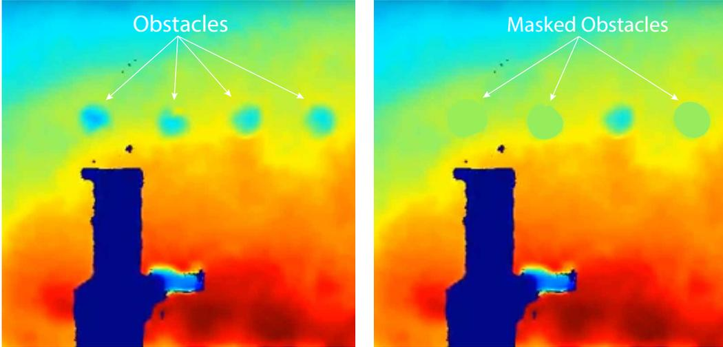
Figure 10: Example of masked image  $\tilde{x}_t$ . The left image is an example of  $x_t$  and the right image is the corresponding masked image  $\tilde{x}_t$ . Specifically, the second to the right most obstacle is the selected obstacle and other 3 obstacles are masked.
