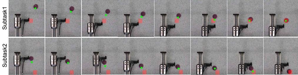
Figure 6: Single leg manipulation results, showing one trial of “Single obstacle with sequential tasks”. The red shaded boxes are the obstacle targets. The green dots are the predicted post-excavation locations of obstacles after the leg performs an excavation at its location.
