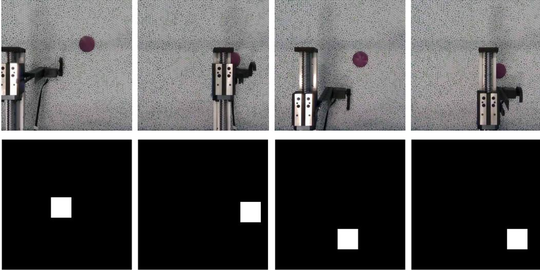
Figure 9: Additional examples of image representations of excavation actions. **Top:** RGB images of robot excavation actions. **Bottom:** The corresponding image representations of robot excavation actions.
