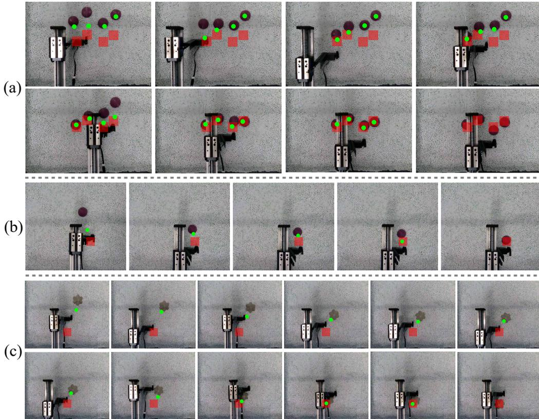
Figure 11: Single leg manipulation experiment results: (a) is Multiple obstacles ( $K = 4$ ), (b) is “Single obstacle with single tasks,” and (c) is “Unseen obstacle.” In the above, red shaded areas are target areas. The green dots are the prediction of post-excitation locations of obstacles after the leg performs the action.
