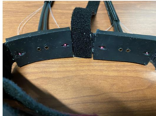
Figure C.1: *Left*: Schematic of functional near-infrared spectroscopy probe. Sources labeled S; detectors labeled D. *Right*: Picture of wearable headband used by each participant, showing the two optical probes. This band is placed on the user’s forehead.
