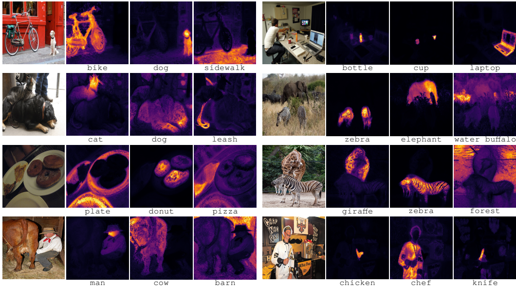
Figure 3: Vision-language alignment of text concepts and dense visual representations. Concepts present in the image are embedded independently by the text encoder and then projected onto the representations of each patch within the image. The images are processed at a resolution of 896 \times 896 pixels, corresponding to 4\times the training resolution. The alignment is performed on LAION-400M using a ViT-B/14 as the vision tower.
