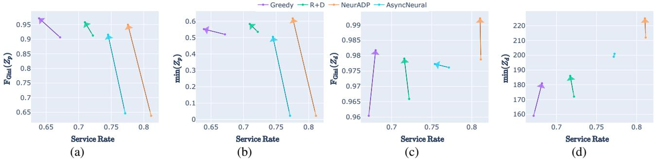
Figure 2: Change in efficiency and passenger-side fairness (with (a)  $F_{\text{Gini}}$  and (b)  $\min$ ) as well as driver-side fairness (with (c)  $F_{\text{Gini}}$  and (d)  $\min$ ) when Simple Incentives are used. The arrows show the best improvement for each algorithm metric while limiting SR to remain above 95% of the initial value. Optimal point is to the top-right (high fairness & high service rate).
