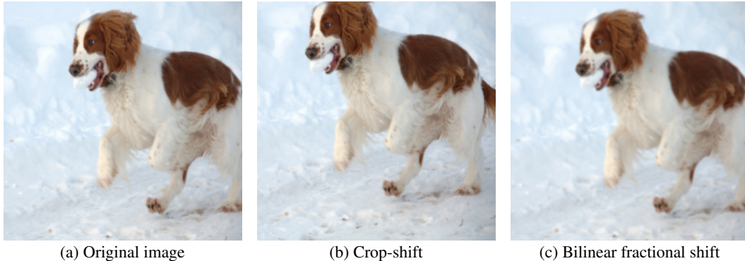
Figure 4: Visualization of realistic shifts. (a) Original ImageNet [12] validation-set image — 224 \times 224 center crop of the original 256 \times 256 image. (b) Crop-shift of the original image of 16 pixels in the horizontal and vertical axes. The cropped area is shifted by 16 pixels with respect to the cropped area in the original image. (c) Bilinear fractional shift of 0.5 pixels in horizontal and vertical axes. We use a 226 \times 226 center crop of the original 256 \times 256 image and simulate a fractional-pixel shift using a grid-sample with a fractional offset.
