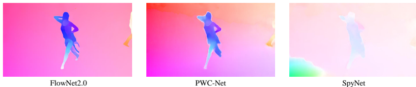
Figure 12: Optical flow quality comparison. This figure highlights the quality of optical flow estimated with various optical flow estimation networks. The optical flow estimated with FlowNet2.0 (Ilg et al., 2017) contains sharp boundaries with minimal noise. Whereas, the optical flow estimated through PWC-Net (Sun et al., 2018) and SpyNet (Ranjan and Black, 2017) contains a significant amount of noise.
