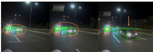
Figure 5. Visualized detection results of FCVL at night with light variations. The model is trained on only daylight samples with the proposed FCVL.
